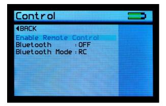
The Control Screen is used to configure the instruments Bluetooth parameters to the user's preference. Pressing the Up and Down buttons navigates through the options, pressing the Enter button selects that option.
