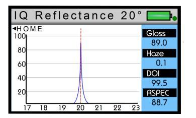
The same paint applied to two panels, the second system has orange peel/waviness which is due to incorrect application setting on spray gun. RSPEC is shown by the red line.4
