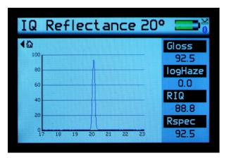
The goniophotometric profile and data for the last 20° measurement will be shown. Measurements can be taken whilst in this screen and the display will be updated.
