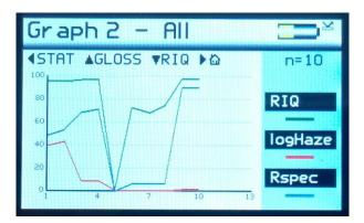
Pressing the Up / Down buttons IQ data can be displayed either all together or individually.
