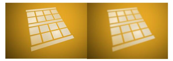
When viewing the reflection of a strong light source in a surface with high haze the image "blooms" and has a bright halo around it.
