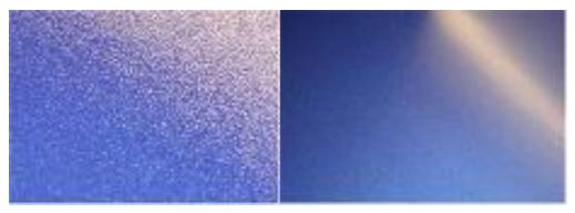
Example test panels with low and high DOI values. Orange peel, texture, flow out and other key parameters can be assessed in coating applications where high gloss quality is becoming increasingly important.
