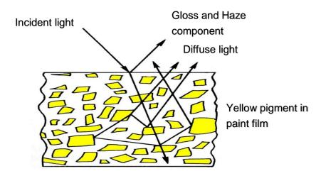
The Rhopoint IQ compensates for reflection from within the coating for highly reflective pigments, metallic coatings and speciality pigments, allowing the haze of any painted surface to be measured.
