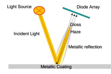
The Rhopoint IQ captures compensation information from a region adjacent to the haze measurement angle, this means it can be used on metallic coatings which reflect light directionally
